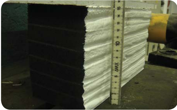
After 1000 cycles there was no visible or physical deterioration of the Flexi®-Coat.
