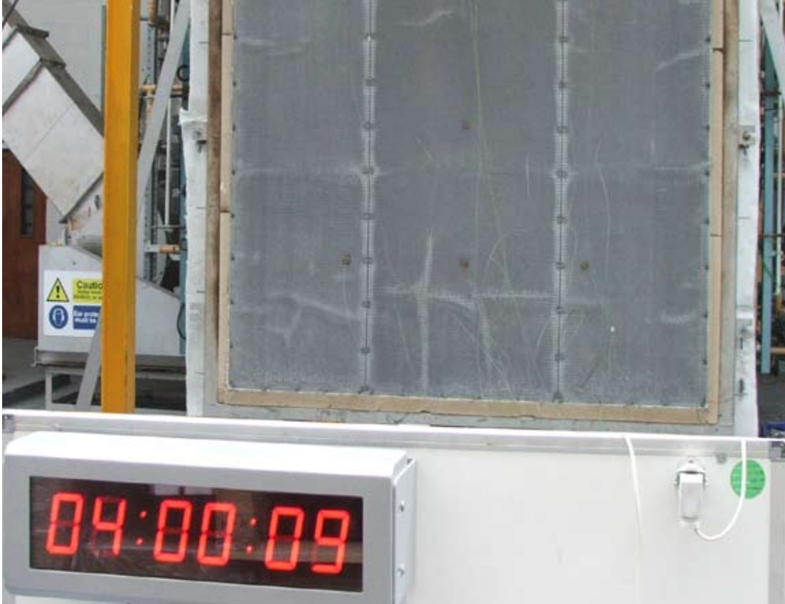
The picture above shows Promat DURASTEEL® wall being fire tested to E240. Below are examples of Promat DURASTEEL® UK and International certification.
