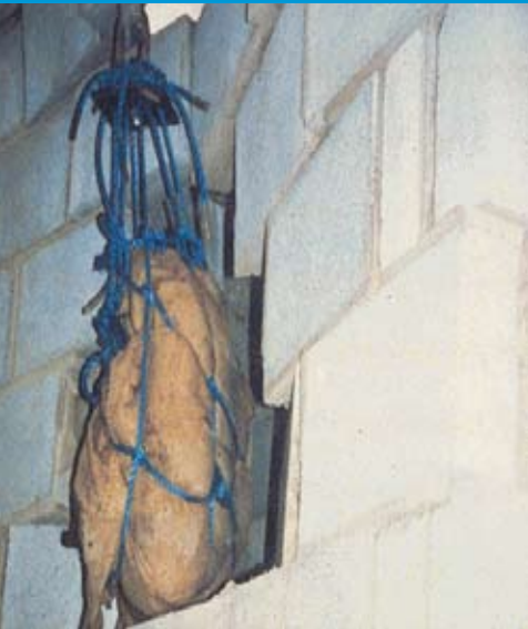
The picture right shows a Promat DURASTEEL® wall undergoing impact following a fire test. The picture above shows a concrete block wall undergoing similar testing.
